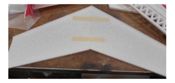
2) Position wing cores on shucks on top of wax paper tape core together and glue together.
