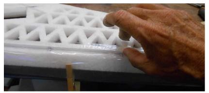
20) Using the tip of covering iron, iron the covering to the trailing edge of the wing.
