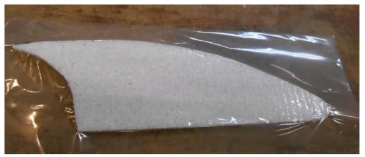
Iron to one side then flip over and trim as shown. Finger cuts are necessary as the covering does not shrink or stretch like most iron on coverings.
