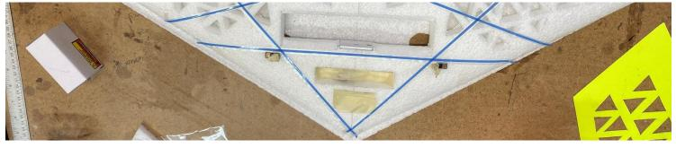
12)Spray light coat of 3M77 contact glue on the airframe. Let flash off for 1 hr. or until it is no longer sticky, just slightly tacky.
