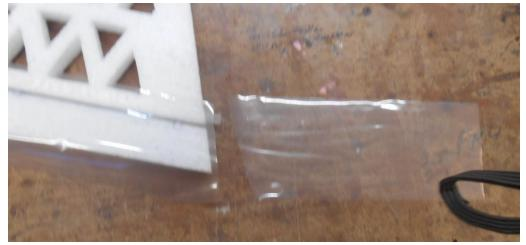
Shape covering and wrap air brake from both sides.
