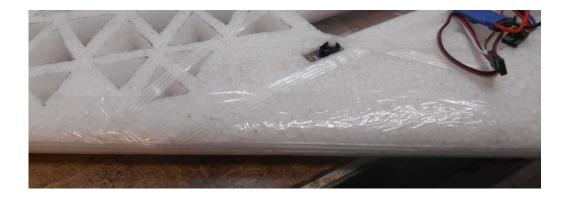
27)Repeat process on bottom of other wing then top of both wings. Cut holes in top covering for servo.
