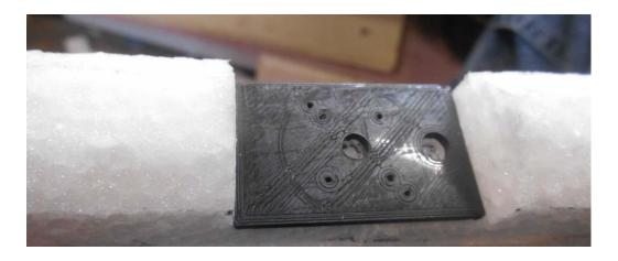
8)Clear holes of excess glue for motor wires.
