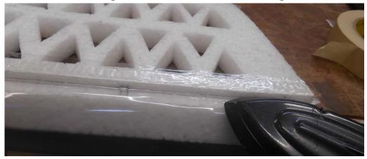
22) Now side wing forward, so alerion is flat. Smooth the covering on to alerion with your finger, then iron covering smoothly on alerion around the trailing edge and on to the other side.
