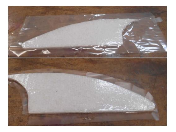
34)Position Indoor tips as shown to ensure you make a right and left. Again cover both sides of of winglets.
