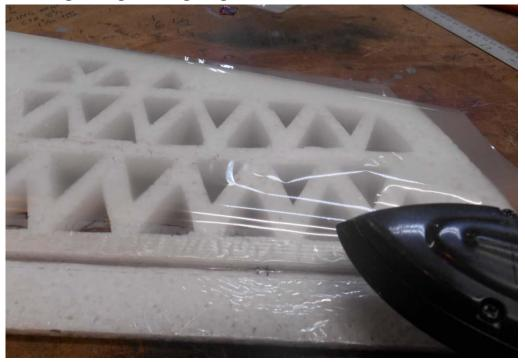
Flip wing over and trim covering at leading edge of wing leaving approximately 1" to wrap around leading edge
