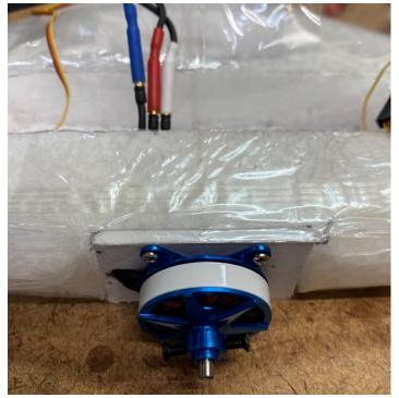
42) Connect to ESC and RX, connect to battery and make sure motor is turning CCW. If not switch any two of the motor wires.
