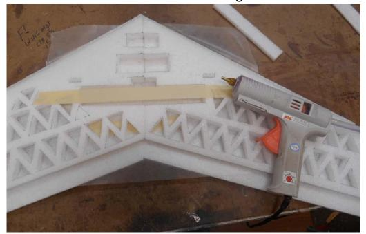
3) Draw lines on the leading edge of prop slot top and bottom and cut bevels to ease the transition of air to prop. Use a triangle to make them square with the centerline of joined wing halves and to check the squareness of the motor mount notch
