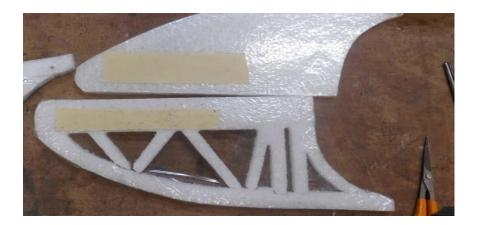
37) Apply stick back velco be sure to the pices marked wing go on wing and winglets go on winglets.(There are four pices marked winglets so you can change between indoor and outdoor winglets)
