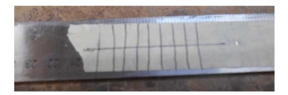
3) Place aileron next to the trailing edge of the wing and place tape tabs to mark the location of hinges at ½",5" 6",11", and 15 ½". The one at 5" is the location of the control horm
