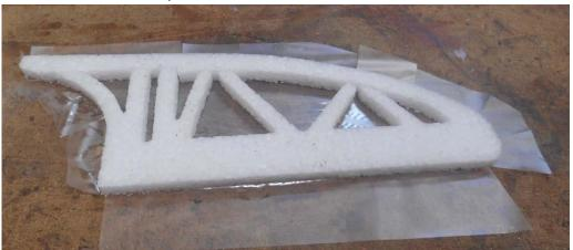
Note fingers cut to facilitate wrapping around curved surface with as few wrinkles as possible.
