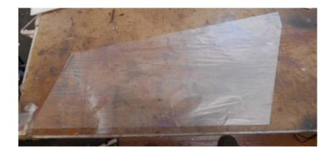
26)Lay covering on wing leaving approx. ½" margin at tip and 3" at center. Align with trailing edge of wing.
