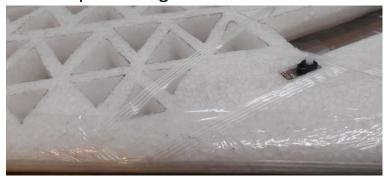
28)Cut covering over prop slot as shown and iron to foam in prop slot.
