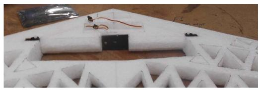
11)Push servos into the wing, so the tops of the case are level with foam. Tape tops of servos and rx and battery compartments to keep glue off.
