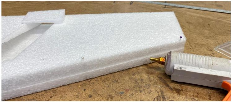
5) Trim ½" off each end and insert wing. And cut hole to clear battery connection.
