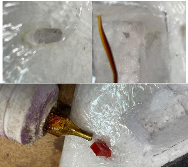
43) Make a channel for battery connection foam and hot glue in place.
