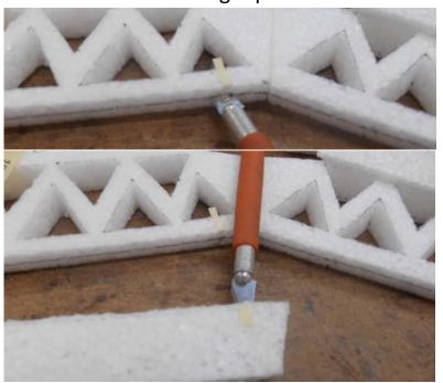
5) Insert c/a hinges into slots cut in the alerions and work them into slots in the trailing edge of the wing.
