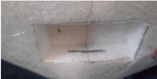
41) Glue in nose weight with foaming glue to keep weight from cutting its way out of foam.
