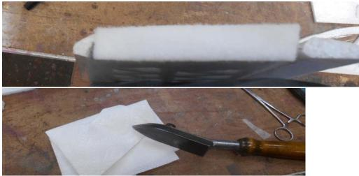
Wipe hot iron on paper towel to clean off most of glue then use alcohol to clean off any residue.
