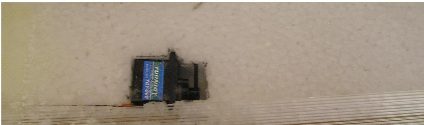
Glue the servo in. Give the wing a coat of 3m77™ then apply 1-inch strapping tape to the wing on the leading edge, over the spars, and on the trailing edge. ( top and bottom)
