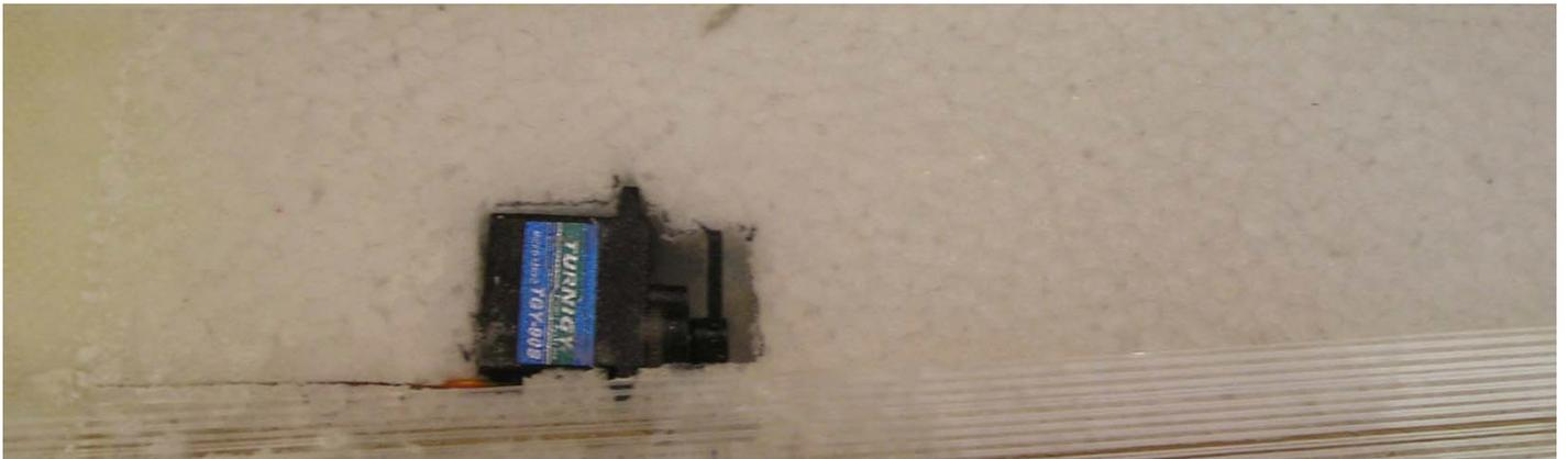
Glue the servo in. Give the wing a coat of 3m77™ then apply 1-inch strapping tape to the wing on the leading edge, over the spars, and on the trailing edge (top and bottom).
