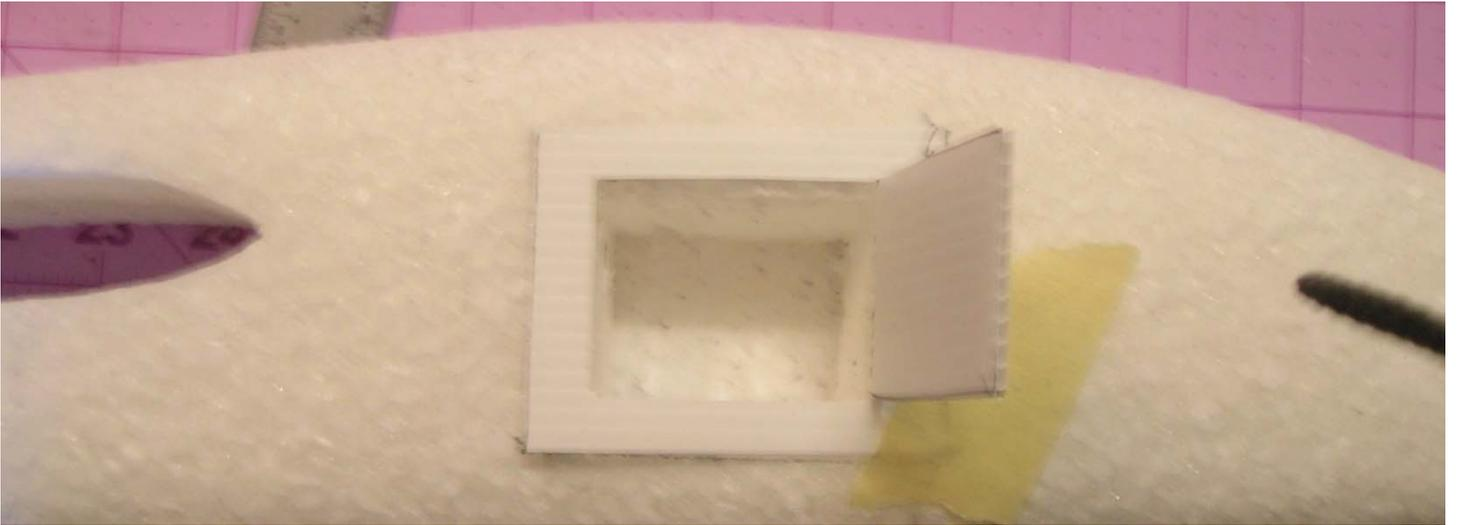
Make pockets for you gear as necessary. Cut a recess for the wing servo wires and extensions to reach the RX. Once the gear is installed tape, the fuse halves together and make sure the elevator linkage is bind free. You will need to cut a recess at the rear of the fuse for the elevator control horn.
