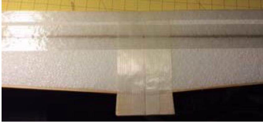
Tape the center section of the wing front to back to distribute the load where it will be glued into the fuse.
